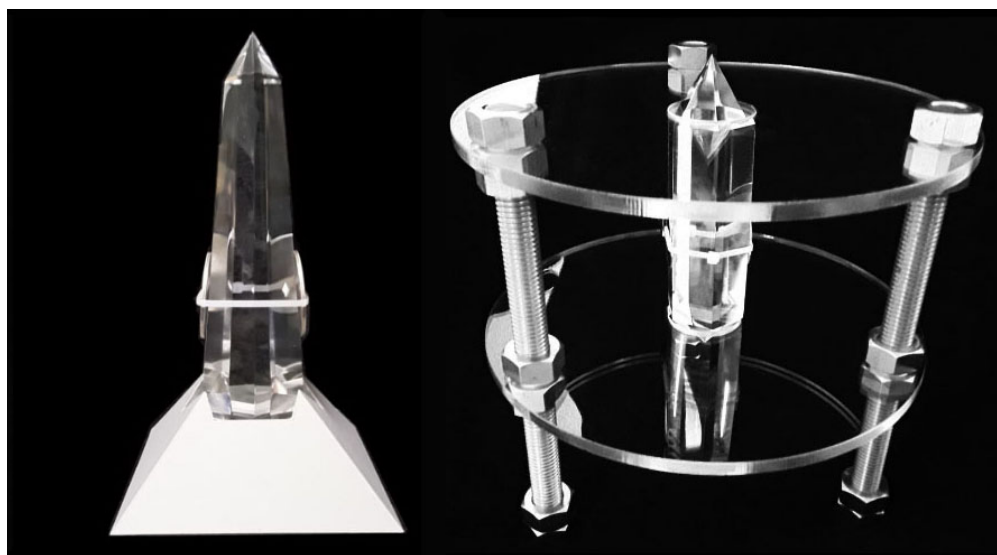
Two configurations to support the crystal with pure silver electrodes
